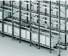
'Jay' Pallet shuttle systems are a semi-automatic or Fully automatic storage solutions for handling goods inside channels similar to Drive-In systems. Radio Shuttles & Satellite Shuttle systems are multi-deep storage system equipments in which radio(satellite) moves within the rack, thus eliminating the need for forklifts, to reach inside the lanes.
